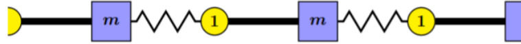
Figure 3.6: The resulting monatomic lattice in the stiff spring limit for a general dimer where all masses have the value 1 + m .
