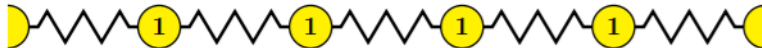
Figure 3.3: Under the equal mass limit, the mass dimer from Figure 1.2 turns into this monatomic lattice.
